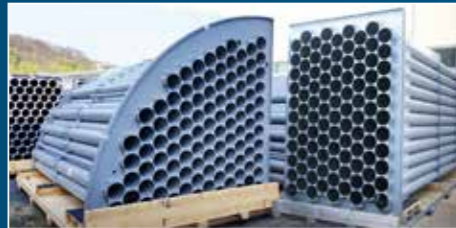
Ready-to-install tube bundle including several redundant grounding of the tube bundle ends with carbon inserts.
