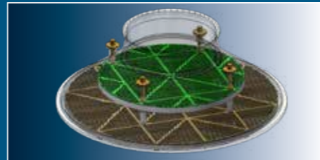
Two-level thermoplastic upper gas distribution. Plates with freely definable hole pattern for optimum gas distribution.
