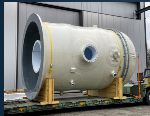
Separator made of KERAVERIN® PTFE-M / FRP. Dimensions DN 3100 x 5639 mm.
