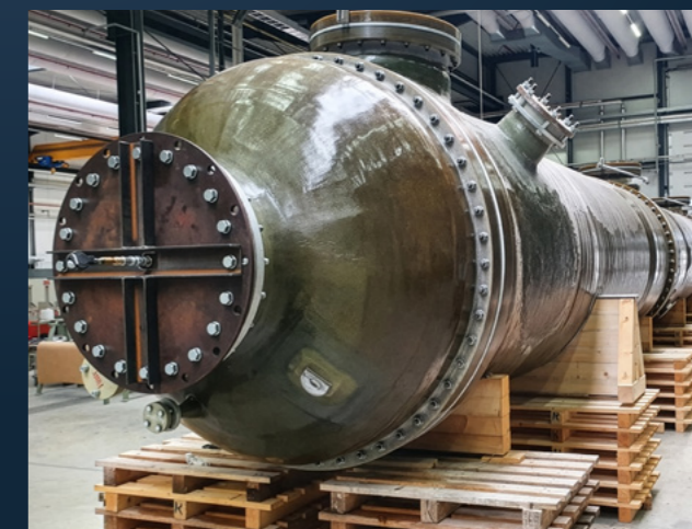
HCl absorption column made of KERAVERIN® PTFE-M / FRP. Dimensions DN 1700/2300 x 31460 mm.
