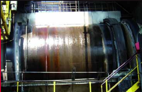
Left: Water-cooled rotary kiln of a hazardous waste incinerator.
