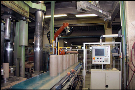
Fig. 1 a (left) and b (right): Dry pressing of center runners and runner bricks
