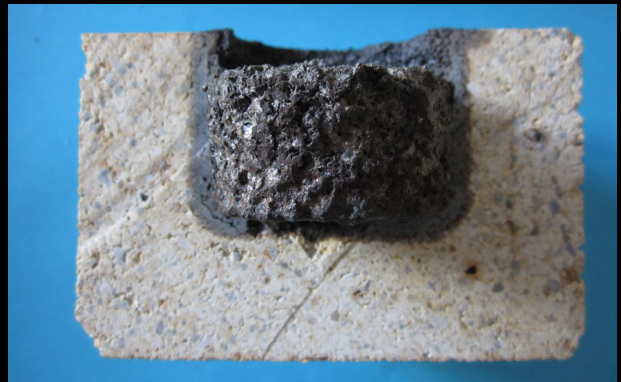
Fig. 4 a (left) and b (right): Crucible test on improved 1st generation high-alumina (bauxite) material with steel P 900, 2 h at 1530° C, without (a) and with (b) residual steel bone
