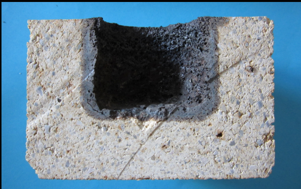
Fig. 4 a (left) and b (right): Crucible test on improved 1st generation high-alumina (bauxite) material with steel P 900, 2 h at 1530° C, without (a) and with (b) residual steel bone
