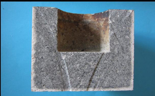
Fig. 10: Crucible test on 99% alumina material containing Nitride Steel P 900, 2 h at 1530° C, without (a) and with (b) residual steel bone. Absolutely no wetting. Consider the crucible is discolored from outside through the test and the grey color inside is original and not caused by the steel test.
