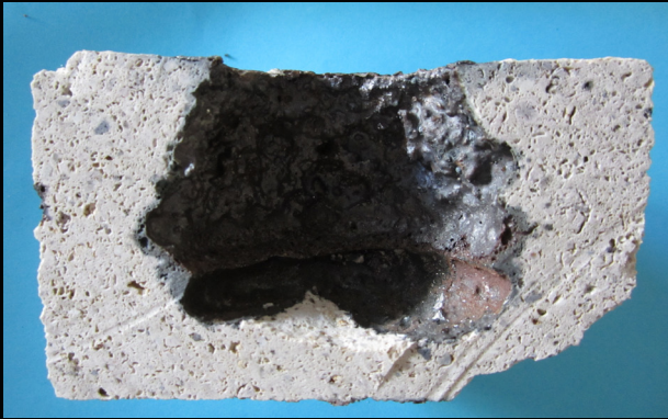
Fig. 3 a (left) and b (right): Crucible test on standard fireclay material with steel P 900, 2 h at 1530 °C, without (a) and with (b) residual steel bone
