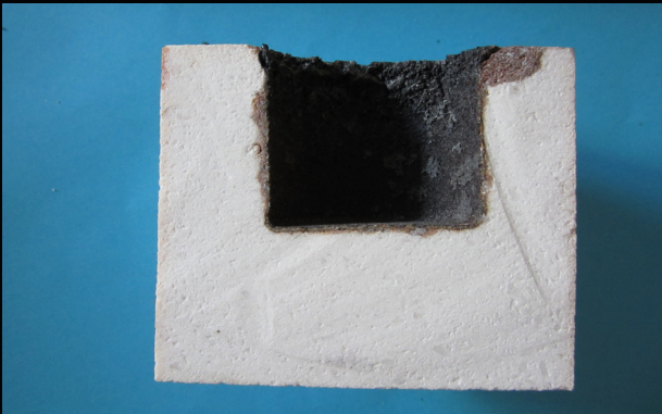
Fig. 8 a (left) and b (right): Crucible test on 99% alumina material with steel P 900, 2 h at 1530° C, without (a) and with (b) residual steel bone
