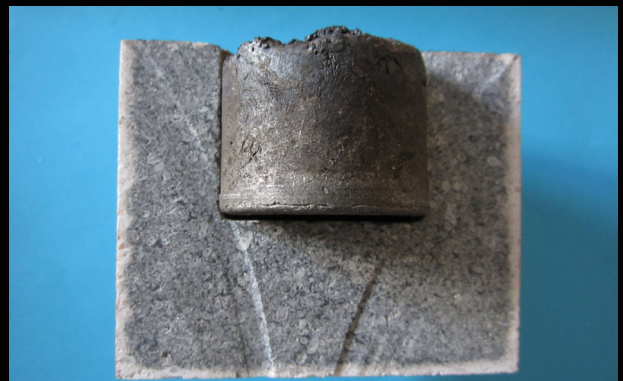
Fig. 10: Crucible test on 99% alumina material containing Nitride Steel P 900, 2 h at 1530° C, without (a) and with (b) residual steel bone. Absolutely no wetting. Consider the crucible is discolored from outside through the test and the grey color inside is original and not caused by the steel test.
