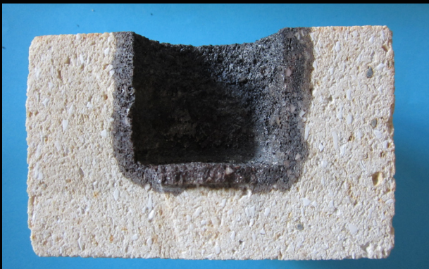
Fig. 5 a (left) and b (right): Crucible test on improved 2nd generation high-alumina (corundum) material with steel P 900, 2 h at 1530° C, without (a) and with (b) residual steel bone
