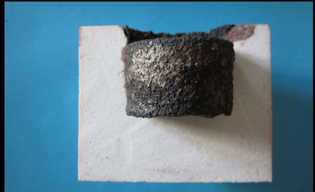
Fig. 8 a (left) and b (right): Crucible test on 99% alumina material with steel P 900, 2 h at 1530° C, without (a) and with (b) residual steel bone
