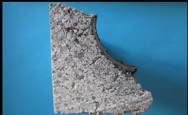
Fig. 5 a (left) and b (right): Crucible test on improved 2nd generation high-alumina (corundum) material with steel P 900, 2 h at 1530° C, without (a) and with (b) residual steel bone
