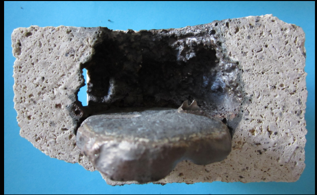
Fig. 3 a (left) and b (right): Crucible test on standard fireclay material with steel P 900, 2 h at 1530 °C, without (a) and with (b) residual steel bone
