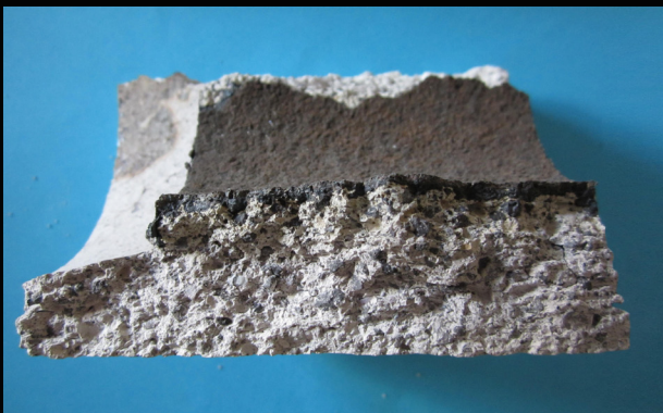
Fig 6 a and 6 b: Bauxite runner brick after use
