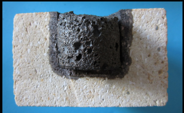
Fig. 5 a (left) and b (right): Crucible test on improved 2nd generation high-alumina (corundum) material with steel P 900, 2 h at 1530° C, without (a) and with (b) residual steel bone
