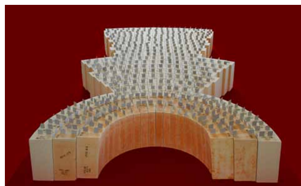
Above: Blast furnace bottom segment
