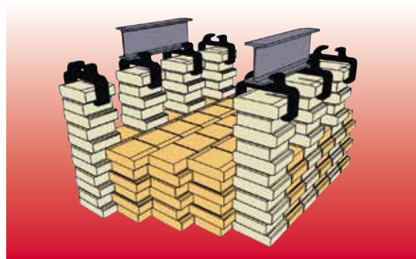
Above: Dry suspended ceiling for aluminium melting and holding furnace
