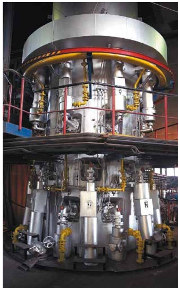
Right: STEULER-KCH lines cathode shaft furnaces in the copper industry with SiC materials.
