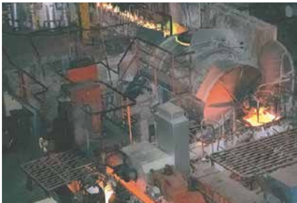
Above: Holding furnace in a continuous casting plant for copper.
