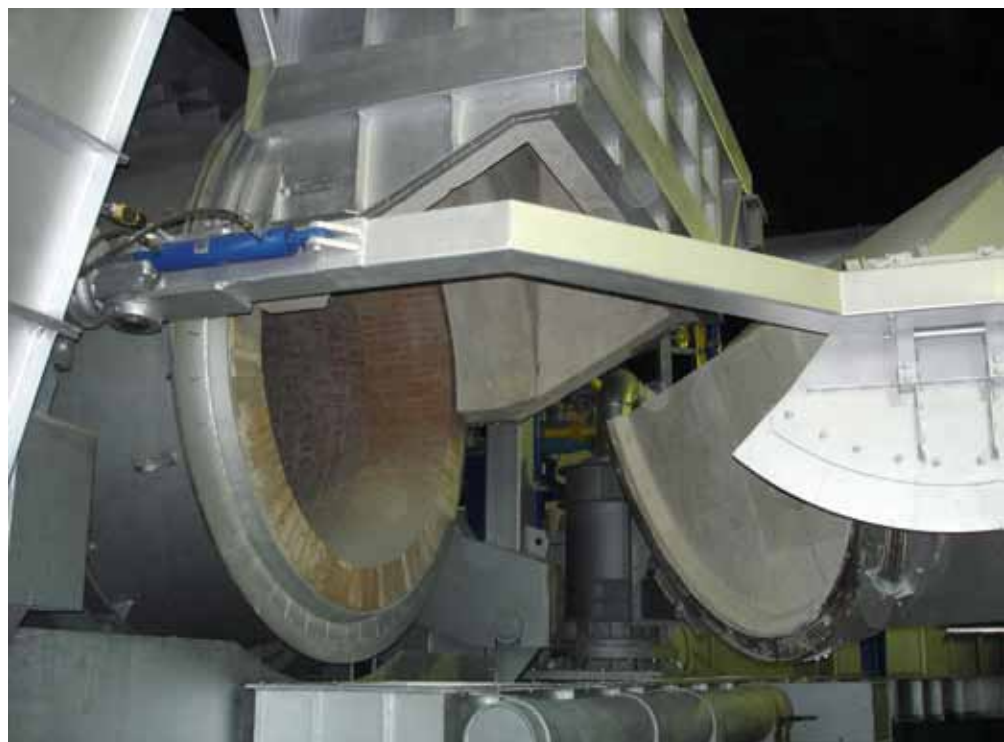
Photo on the right: Rotary tilting furnace for recycling under usage of salts
