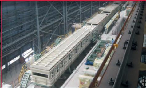
**Above:** Construction of a completely prefabricated Polypropylene Tank system for a steel band pickling plant.
