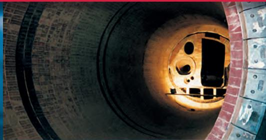
**Above:** View into a refractory lined toxic waste incineration furnace.
