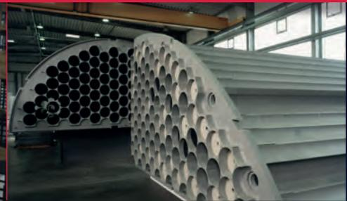
**Above:** Tube bundles for wet electrostatic filter for a Gas Cleaning Plant made from flame retardant polypropylene.
