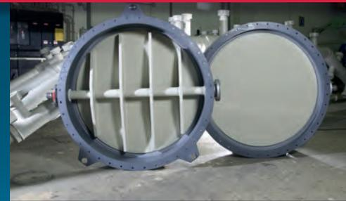
**Above:** Throttle valve with actuator.
