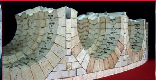
**Above:** Refractory inlets of a hot blast tuyere for a steel blast furnace.
