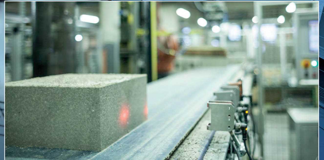
Opto-electronic dimensional inspection in ceramic brick production – ensuring that everything fits afterwards.
